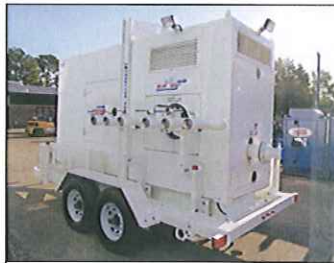
Photo: Thompson Pumps Water pumps—like the one pictured above—can provide up to 1,850 GPM and head up to 670 feet.
